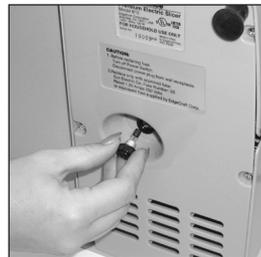
**Figure 10. Replacing the fuse located underneath motor housing.**
