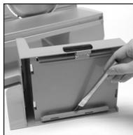
Figure 6. Lubricating the food carriage guides.
