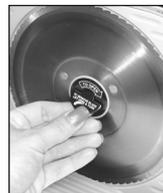
Figure 7. Turn the screw clockwise for blade removal.
